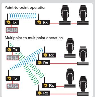
W-DMX is unique in its use of certain advanced radio techniques which are more often found in mobile phone and military communications. Rather than using fixed frequency channels, W-DMX uses adaptive frequency hopping technology (as well as TDMA and GFSK technqiues) to continually check for interference and to rapidly move operation over to clear radio channels. The frequency hops occur one thousand times every second to ensure smooth, efficient and robust operation
